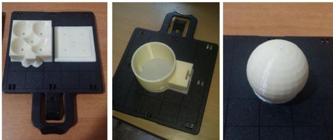
Fig.4 Sensor array, laser frame and laser holder after rapid prototyping
